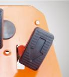
HST models employ a two pedal system for forward and reverse with smooth engagement, acceleration and deceleration. Pedal pressure is minimized which reduces operator fatigue during long hours of use and when doing repetitive tasks.
