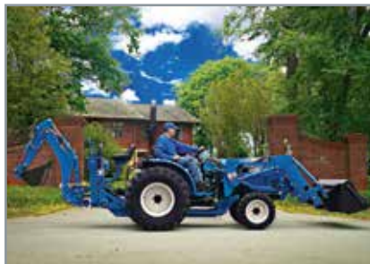
Optional quick attach backhoe Remove or attach in seconds. With 76" digging depth, 2,817 lbs of digging force and 180° swing arc, it outperforms other in its class.
