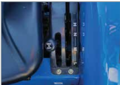
Simple gear range selections Select your gear range or 2WD/4WD with simple move of the levers.
